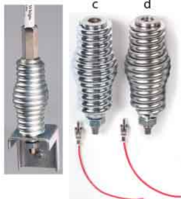
Heavy Duty Spring Mount Highly recommended to help reduce whip breakage.
