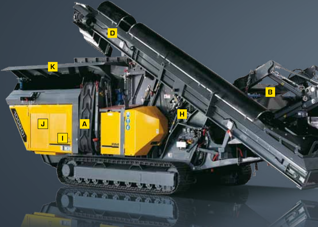
Vibro feeder The innovative single-piece vibro feeder with integrated prescreening means that material is fed into the crusher in an optimum manner.
