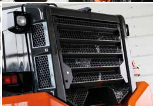
New rear grill protects radiator compartment.
