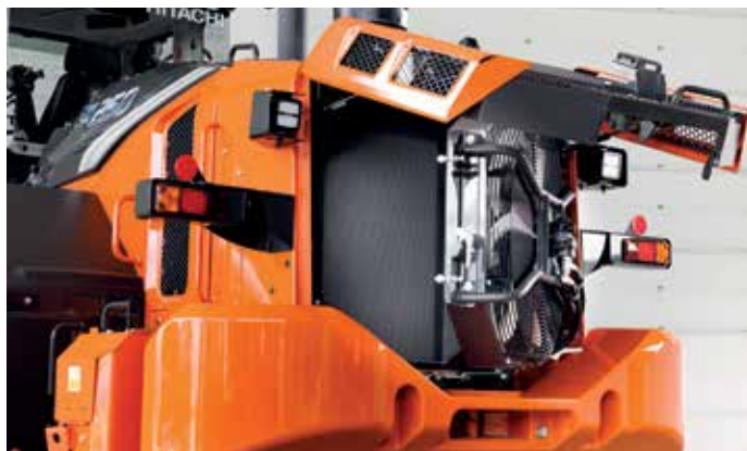
Intelligent fan operation system prevents radiators clogging.
