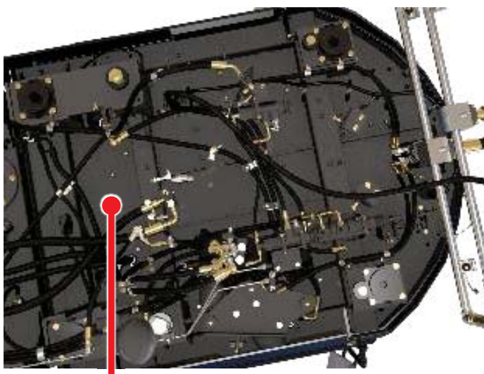
Rubber clamps for pilot hoses and additional noise absorber under the cab floor
